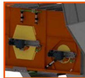
Premium Windshifter splits materials in three fractions and is suitable for all kinds of waste. The HuMeij Premium Windshifter (PW) is a unique air classifier with a range of both indoor and outdoor possibilities. The machine is delivered in efficient sub-assemblies for easy shipment and handling.
